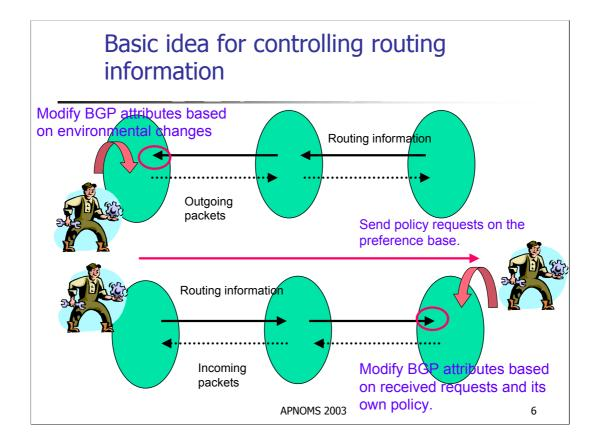
As shown in this figure, we are difficult to know the behavior of spreading inter-AS routing information or to control it to fit policy as the originator intends at the inter-AS level. BGP defines several attribute parameters for controlling policy, but policy cannot utilize these parameters effectively if the policy is controlled on a single router in an AS using only static low level configuration primitives.
