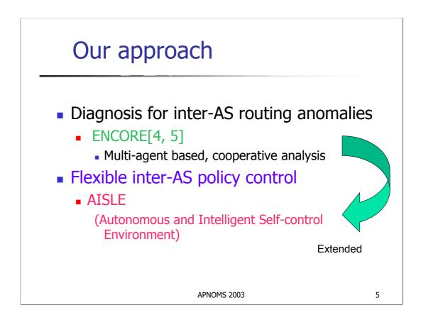
These problems require that autonomous policy control process should share inter-AS routing information from outside the AS and a cooperative distributed solution should be established. Moreover, intermediate control layer between policy and router configuration is desirable.
