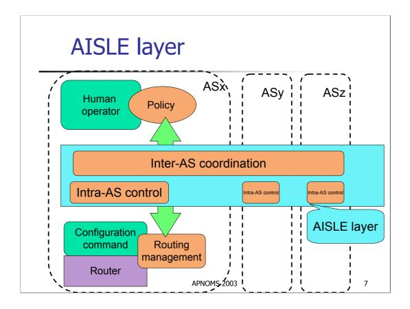
The policy control layer of AISLE is realized as it exists between policy that resides in human operators and router configuration commands. The AISLE layer consists of intra-AS control part and inter-AS control part since each AS is independently managed and a simple centralized model would be difficult to apply. We can assume that an agent can access routing information in its AS because the AS is controlled by the same administrative authority.
