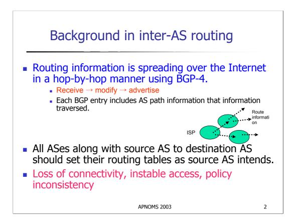
Border Gateway Protocol (BGP-4) [1] is widely used for inter-AS (Autonomous System) routing and has become the current de facto standard. The AS that receives BGP information selects only one route per destination as a best path based on the AS's policy, and passes the information to other ASes. So the routing information spreads among these ASes in a hop-by-hop manner.
