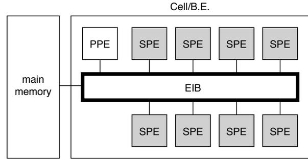
Figure 1. The architecture of Cell/B.E.
