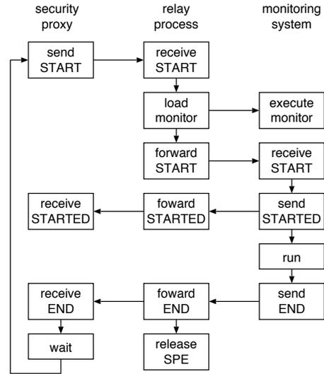
Figure 6. The flow chart of scheduling monitoring systems.
