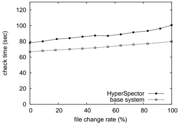
Figure 10: Time for integrity checking in Tripwire.
