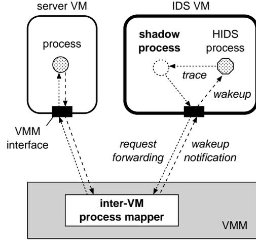
**Figure 5: Process monitoring using the inter-VM process mapper.**
