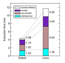
Figure 6. The breakdown of the execution time of each thread in the thread pool (ms).
