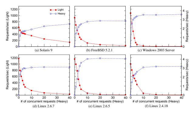
Figure 1. Degradation schemes of various operating systems. (workload 1)
