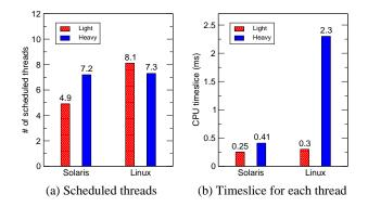
Figure 7. The total number of threads scheduled during execution of each thread in the thread pool and the time slice (ms).
