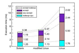
Figure 10. The breakdown of the execution time of each thread in the thread pool in Linux with short time slices.
