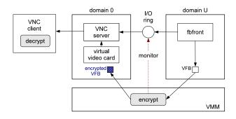
Figure 4. The encrypted delivery of pixel data.
