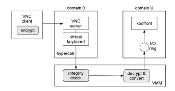
Figure 3. The encrypted delivery of keyboard inputs.
