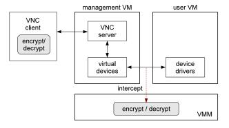
Figure 1. The architecture of FBCrypt.
