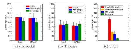
Fig. 10. The increases in CPU utilization during running offloaded IDSes.
