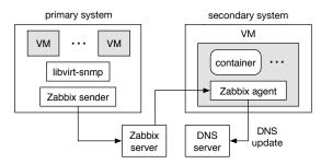
Figure 6: The architecture of VCRecovery.
