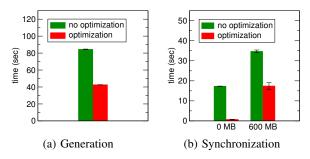
Figure 11: The performance of disk synchronization.
