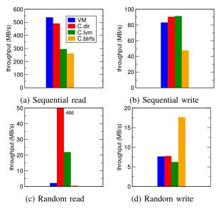
Figure 13: The throughput of file access.
