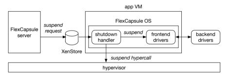
FIGURE 5 Suspending PV devices.
