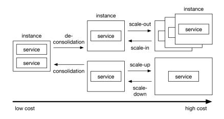
FIGURE 1 Various optimizations of instance deployment.
